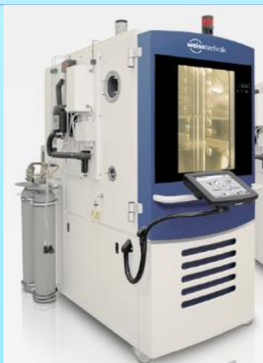
EUCAR Level 6 Environmental Chamber
