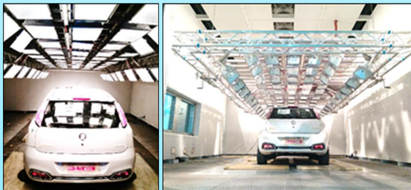
Vehicle inside Drive-in 4-Poster with Integrated Climatic Chamber
